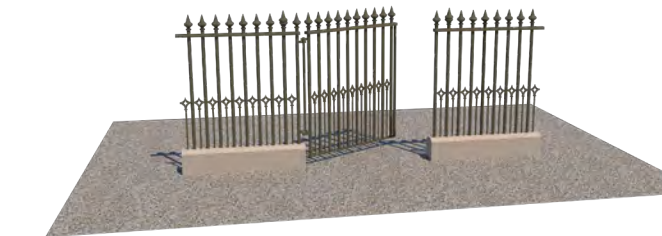
A Proposed Pedestrian Entrance (King William IV Gate) Note : Manual, single leaf gate
