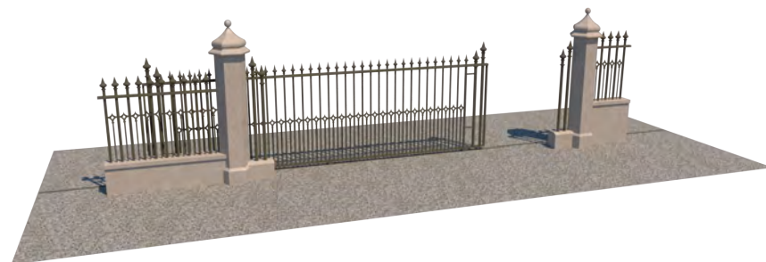
A Proposed Vehicular Entrance (Service Area) Note : Automated sliding gate
